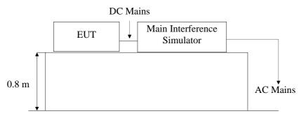
Remark: Combination wave generator and decoupling network are included in test generator.
